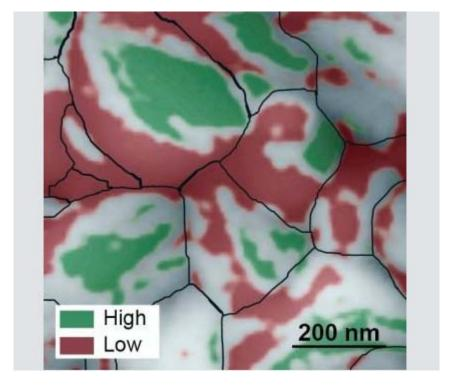
This atomic force microscopy image of the grainy surface of a perovskite solar cell reveals a new path to much greater efficiency. Individual grains are outlined in black, low-performing facets are red, and high-performing facets are green. A big jump in efficiency could possibly be obtained if the material can be grown so that more high-performing facets develop.
